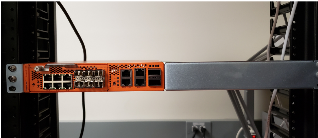
Figure 10 Four-Post Rack Installation (Single Chassis Assembly)
